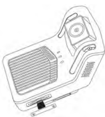
Micro SD card installation
