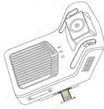
SIM card installation
